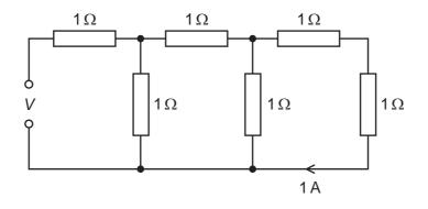
The current passing through the end resistor is 1A.
