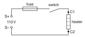
Terminals S+ and S– are the positive and negative terminals of the supply. Points C1 and C2 at either side of the heater are accessible for fault-finding.
